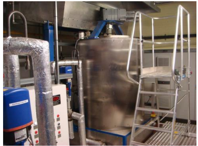
Pellet melting unit with heated holding tank. In front the oil heater.
