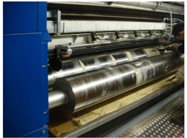
Transfer roller in service and cleaning position
